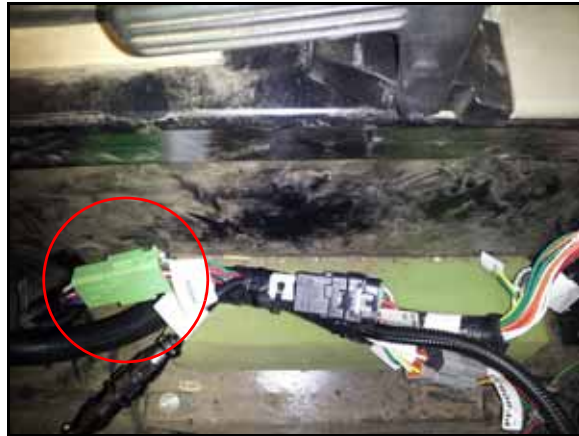
FIGURE 11. Valve Harness Connected to Tee Safety Harness
