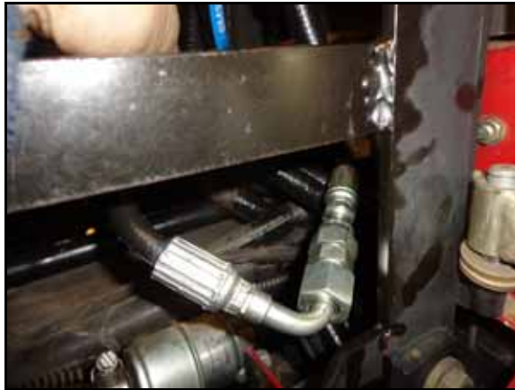
FIGURE 9. Hydraulic Hose Installed on Load Sense Hose
