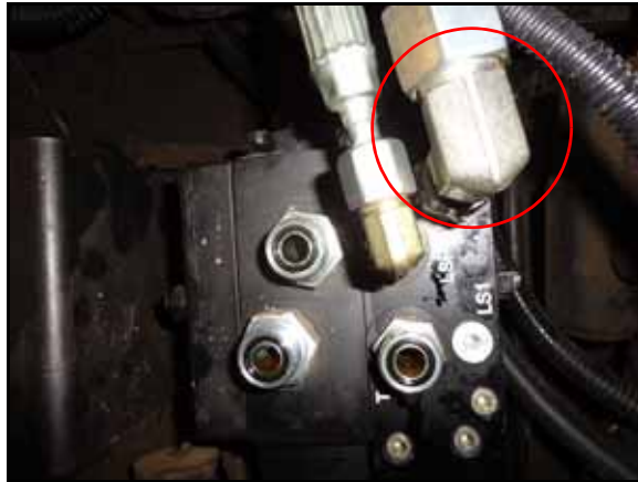
FIGURE 17. Pressure Hose Installed on Steering Valve
