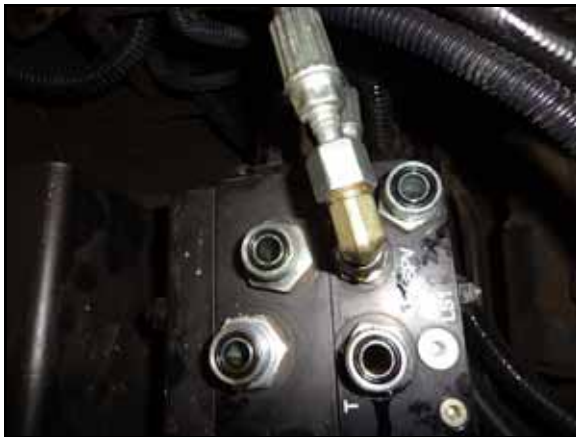
FIGURE 10. Load Sense Hose Installed on SmarTrax Valve
