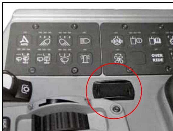
FIGURE 8. Master Switch Installation Location
