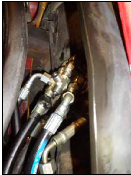
FIGURE 26. Tee Fitting Installed in Left Steering Port
