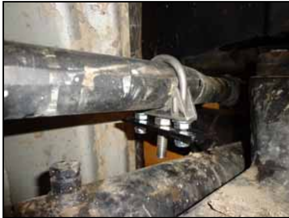
FIGURE 5. Rod Mounting Bracket Installed
