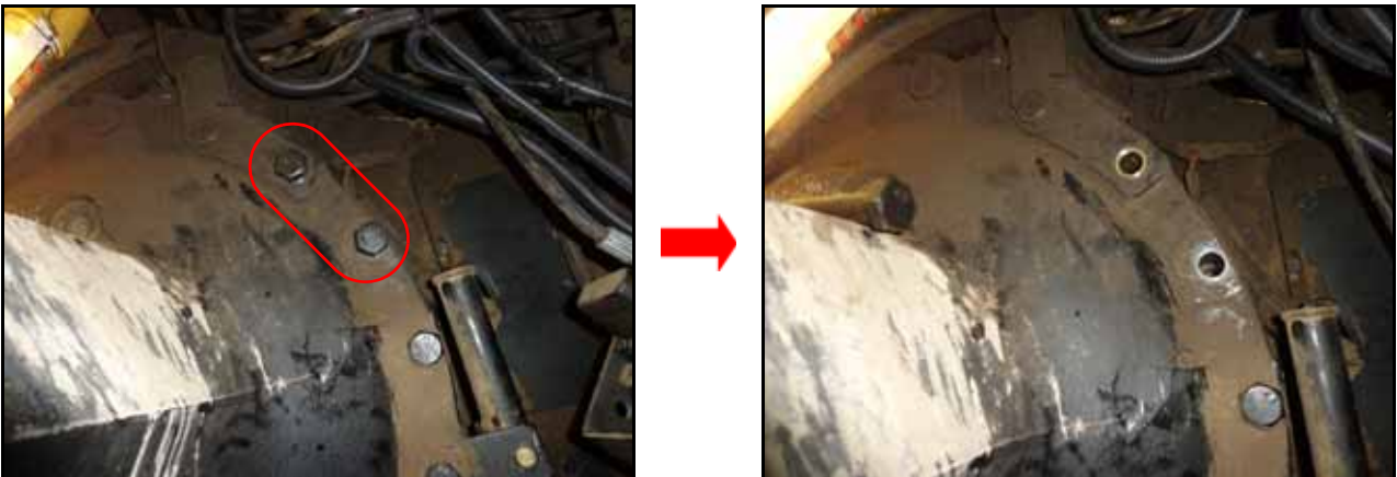
FIGURE 2. Bolts to be Removed
