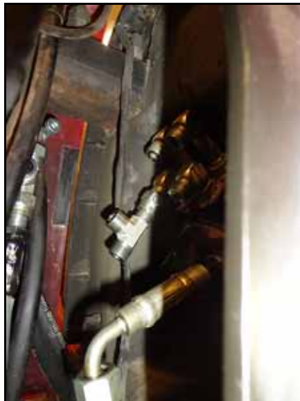
FIGURE 14. Tee Fitting Installed in Pressure Port
