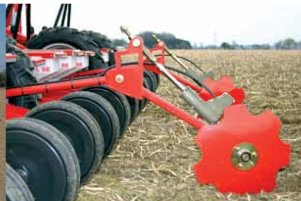
The optional pre-emergence markers assist first spraying operations before seed emergence
