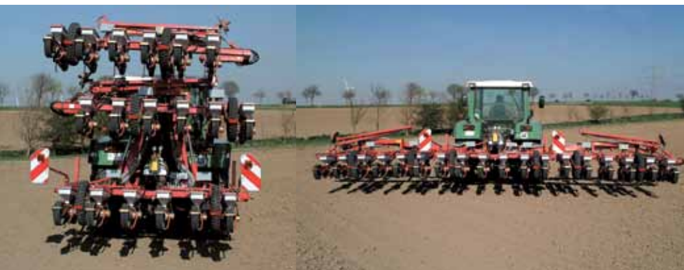
Monopill SE, 9 mtr, 18rows parallel hydraulic folding in transport and working position
